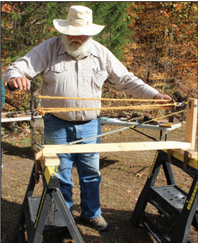
A demonstration is given on how to use a rope making machine.
